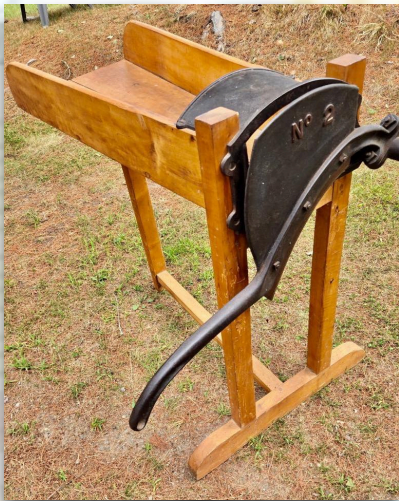
NSHA member, Larry Smith, will refurbish the wooden structure of the corn chopper.
