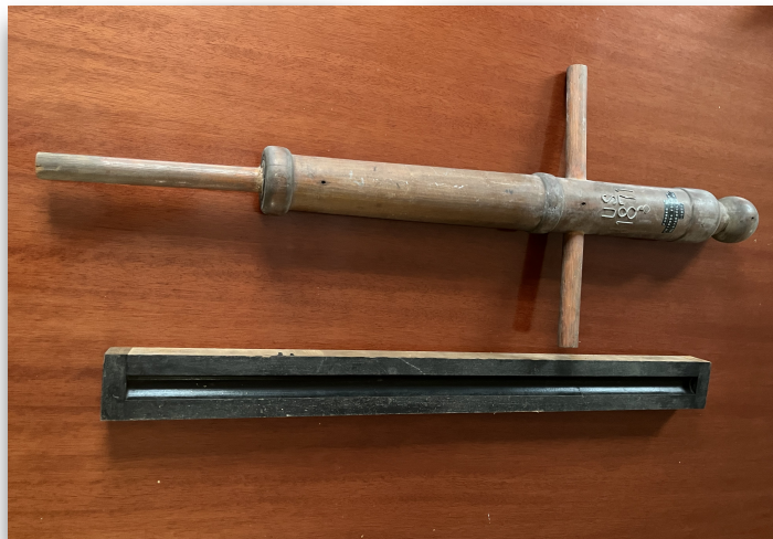
Pictured above is the pattern and core-box used in 1971 to cast the small aluminum cannon that was used in the North Smithfield Centennial parade. Found in Friends Foundry. Donated by the Vadenais Family.
